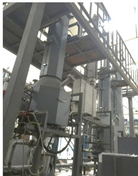
Fig. 1. Schematic view and a picture of the 50 kW th iG-CLC reactor.
